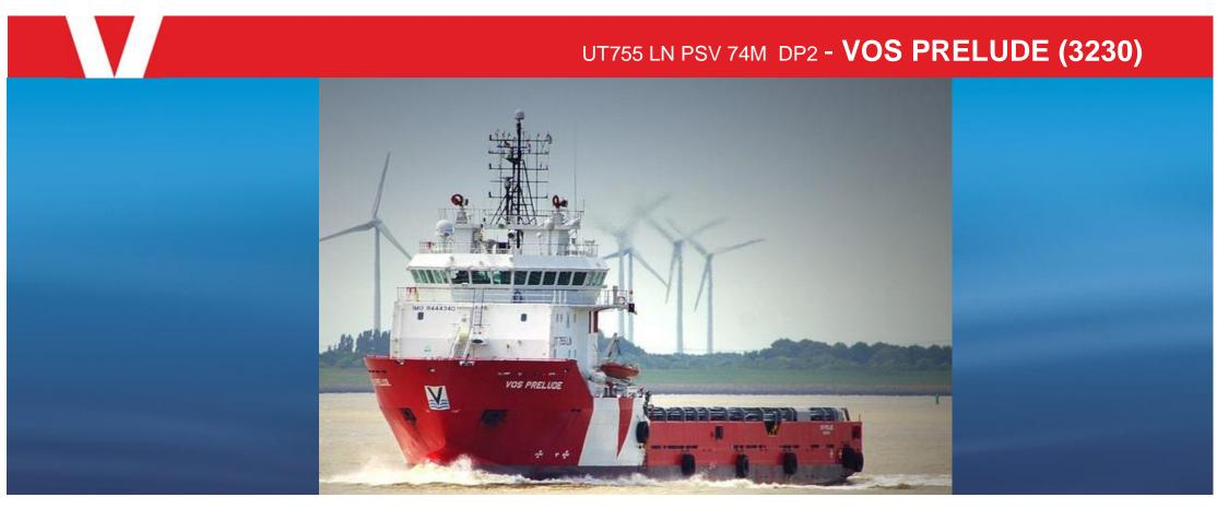
**GENERAL** 2010 Year Built Cochin, India Place of Built Flag Dutch Port of Registry Breskens Call Sign **PBZK** IMO 9444340 Class Lloyds LR  $\, \Xi \,$  100 A1 Offshore Supply Ship, Fire-Fighting Ship 1 (3200m3/h)with Water Spray.LI ★ LMC UMS DP(AA) DYN POS,CLEAN NOTATION 99.99.66 ERN number MMSI 2459690000 PRINCIPAL DIMENSIONS Length Overall 73.6 m 68.3 m Length B.P.P.
