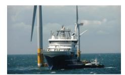
The *Deep Cygnus* is a multifunctional ROV support and construction vessel equipped with a deepwater 150 Te crane and work-class ROV. It is a premier vessel well-suited for playing a key role in any deepwater development project.
